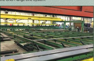
The **Franklin "60" Series** gantries provide up to 60 ft. of length capacity and 75 ft. of travel storage.
