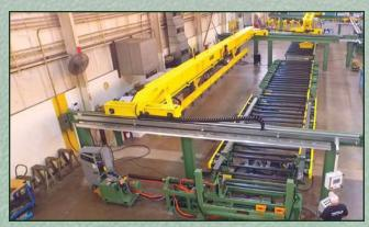
The pass-thru design of the horizontal welding system allows a continuous flow of beam production.
