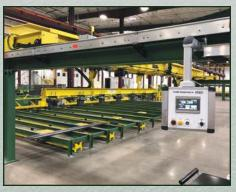
The Franklin auto-flange stacking system provides an efficient handling of hi-volume flange production. Each flange stack can be power transferred directly into the **TS-72 Track Station** gantry pickup zone.
