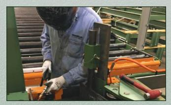
The **TS-72** tack-station system provides hydraulic clamping that pre-fixtures the leading edge of the prefabricated beam.
