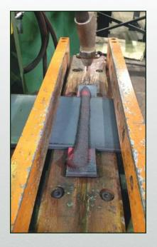
Weld splice station with top acting pneumatic clamps. The Franklin CNC control automatically detects the trailing end splice location within the flange line system.
