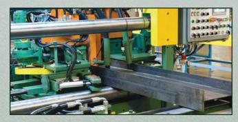
The **Franklin PTW-72** horizontal pull-thru welding system is a highly engineered submerged-arc system.
