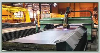
The CNC Plasma Cutting Machine is a highperformance plasma cutting machine with brushless AC servo drives and planetary gear boxes providing positioning speed of 1500 IPM.
