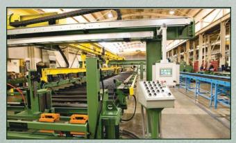
The **Franklin "40" Series CNC Gantry** provides automated pick-and-place loading of finished flanges from the CNC Flange Line System.
