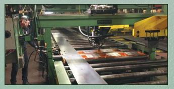
The **WS-72 Web Splice Station** incorporates "pull down" type magnets. The unique design provides adequate power for sheets up to 1/2" while providing the operator an easy-to-access weld area without top clamps.
