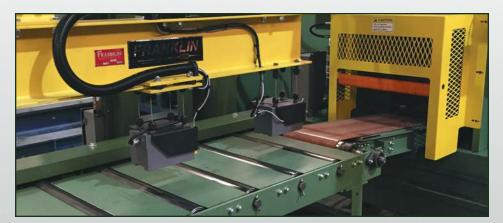
Franklin PF196x20-**CFD CNC Plate** Fabricator is a dedicated plate line for producing connection plates and base plates. The material is moved and positioned by a Servo Carriage and attached to the trail end of the bar by a Hydraulic Gripper.
