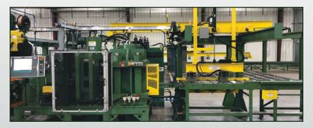
The **Franklin BP5196x20** CNC Plate/Flange Line is a hi-production combination machine for both plate and flange fabrication.
