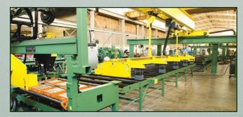
The **Franklin** "20/30" gantry system with dual-row magnets provides web pick and placement at the WS-72 web splice station. Due to various shapes and storage methods, the gantry is controlled manually by a 4-position joystick control.
