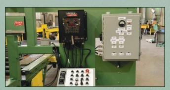
The **WS-72 Control Station** provides the operator control over all conveyors, hydraulic web squaring, and weld speed control. The Lincoln MAX-SA 10 Control is integrated for easy access.
