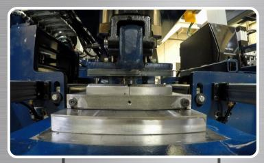
Hi- Speed Shear with 90 ton frame and 3/8" x 8" single cut capacity
